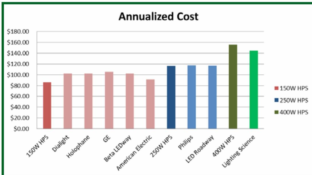
Figure 1. Annualized Cost of HPS Equivalent LED Luminaires
